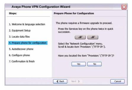
c. Double-press the Services key on the IP Deskphone quickly. Select the Network Configuration menu item. Move the cursor to locate Provision: or (TFTP IP:) in the Network Configuration menu, and then write down the existing address of the provisioning server, so you can return to it after you complete this procedure.
